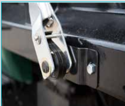
Die-cast aluminum housing, protects springs and strengthens arm joints
