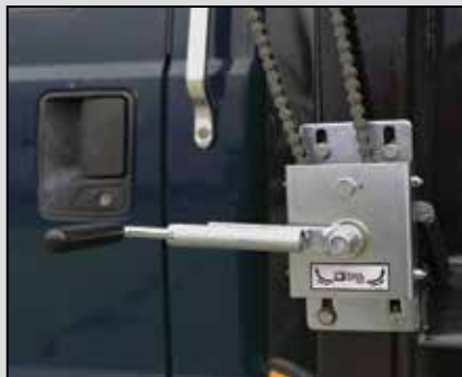
Tarp crank with friction brake (3020293)
