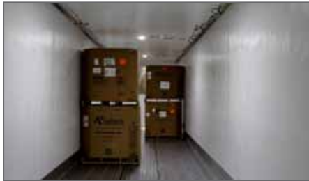
Engineering tests illustrate how ineffectively the traditional arrangement of recessed ceiling dome lights illuminate this 53' insulated reefer trailer.
