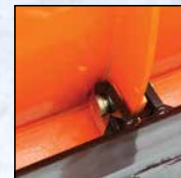
4 Moldboard-to-push frame pivot points have 1-1/4" plated pins through 1/2" ribs with 1/2" bolster plate, bushed to 1-3/8"
