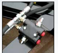
Cushion valve with 1/2" ports protects cylinders from impact loads. Preset at 2000 PSI, adj. from 1500 - 3000 PSI
