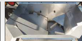
"Hex flow" chute and 24 inch spinner with adjustable baffles for optimal spread pattern
