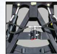
4" HD car and ship channel A-frame supports a 2" plated king pin mounted in a 3" OD x 1/2" wall DOM tube with grease fitting
