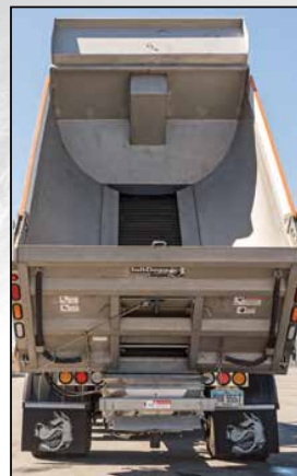
Unique, roll-formed sides and cross member-less design
