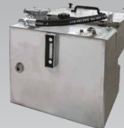
Central Hydraulic System Tank Provides directional oil flow for plow, spreader, and hoist control • Cutting edge, space saving design • In-tank return filter assembly for oil refinement • 4 and 6-Function valve options (additional available) • Bottom ported manifold valving eliminates excessive hoses • 15 and 30 gallon, 304 stainless steel tanks
