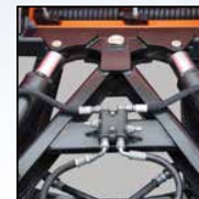
3-1/2" Steel channel A-frame supports a 1-1/2" plated king pin mounted in a 2-1/4" OD x 3/8" wall DOM tube with grease fitting
