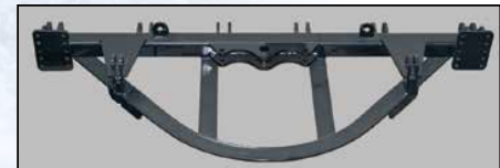
80" Semi-circle has 3-1/2" x 3-1/2" x 1/2" angle, welded to the 3-1/2" x 3-1/2" x 5/16" structural push tube 90" wide
