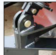
Anchor plates are encased and continuously welded to the push frame providing greater strength
