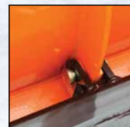
8 Moldboard-to-push frame pivot points have 1-1/4" plated pins through 1/2" ribs bolstered with second 1/2" plate, bushed to 1-3/8"
