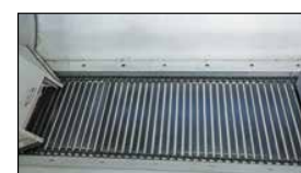
30.25" wide conveyor with 1/2" bars
