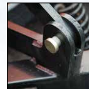
Heavy-duty anchor plates are continuously welded to the push frame providing greater strength
