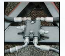
Cushion valve with 1/2" ports protects cylinders from impact loads. Preset at 2000 PSI, adjustable from 1500 - 3000 PSI
