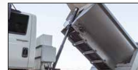
Mailhot® multi-stage, double-acting, nitrided cylinder, trunnion-mounted hoist
