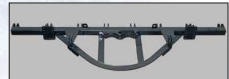
80" Semi-circle has 3-1/2" x 3-1/2" x 1/2" angle, welded to the 4" x 4" x 3/8" structural full length push tube
