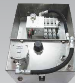
Central Hydraulic System Tank Provides directional oil flow for plow, spreader, and hoist control • Cutting edge, space saving design • In-tank return filter assembly for oil refinement • 4 and 6-Function valve options (additional available) • Bottom ported manifold valving eliminates excessive hoses • 15 and 30 gallon, 304 stainless steel tanks
