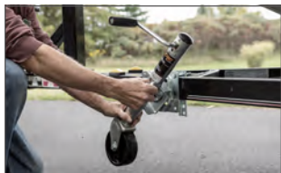
Swivel bracket allows jack to fully swing up during travel
