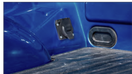
10' routes socket closer to truck cab
