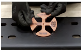
Step 1 - Place Center Locator in the gooseneck hitch ball hole
