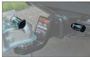
Watertight dust caps prevent internal corrosion
