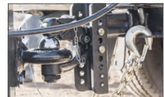
Helps resist total vehicle-trailer separation during a disconnect
