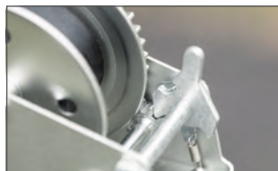
Broached pinion shaft securely engages the pinion gear
