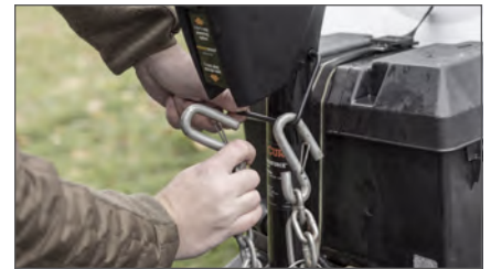
Integrated hanger bracket keeps safety chains out of the way when not in use
