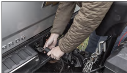
Optional vehicle power connection for no hand cranking or RV battery drain
