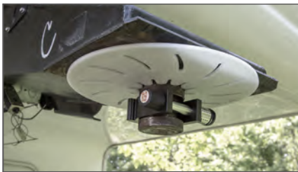
Locks on to 5th wheel kingpin to deter theft of 5th wheel trailer
