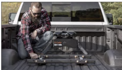
Easily transfer existing hitch from previous truck to new puck-equipped truck
