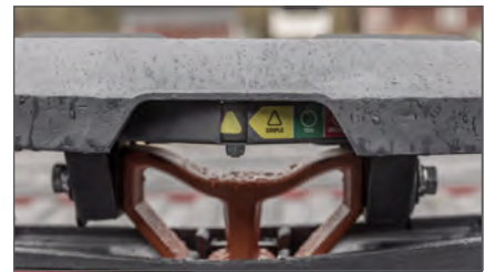
Three-position coupling indicator clearly shows coupling status
