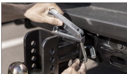
No-tool installation and easy-to-adjust clamp lever (clamp-style)
