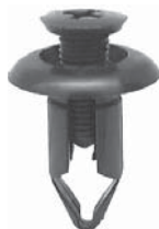
21123 (75867-30120) Black Nylon Rocker Moulding Push-Type Retainer Head Diameter: 18mm Stem Length: 19mm Fits into 8mm Hole Lexus GS350, GS430, GS460 & LS460 and Toyota Camry 2007 - On
