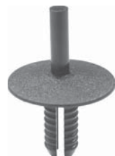
21134 (01553-09431) Black Nylon Front Bumper Push-Type Retainer Head Diameter: 20mm Stem Length: 11mm (Excluding the Pin) Fits into 8mm Hole Nissan Maxima 2004 - On
