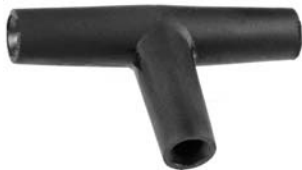
11220 Non-Corrosive Black Polyethylene High-Density Tubing and Hose Elbows Pipe Thread: 1/4" Hose Size: 3/8" I.D.
